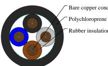
Bare copper conductor Polychloroprene rubber outer jacket Rubber insulation
